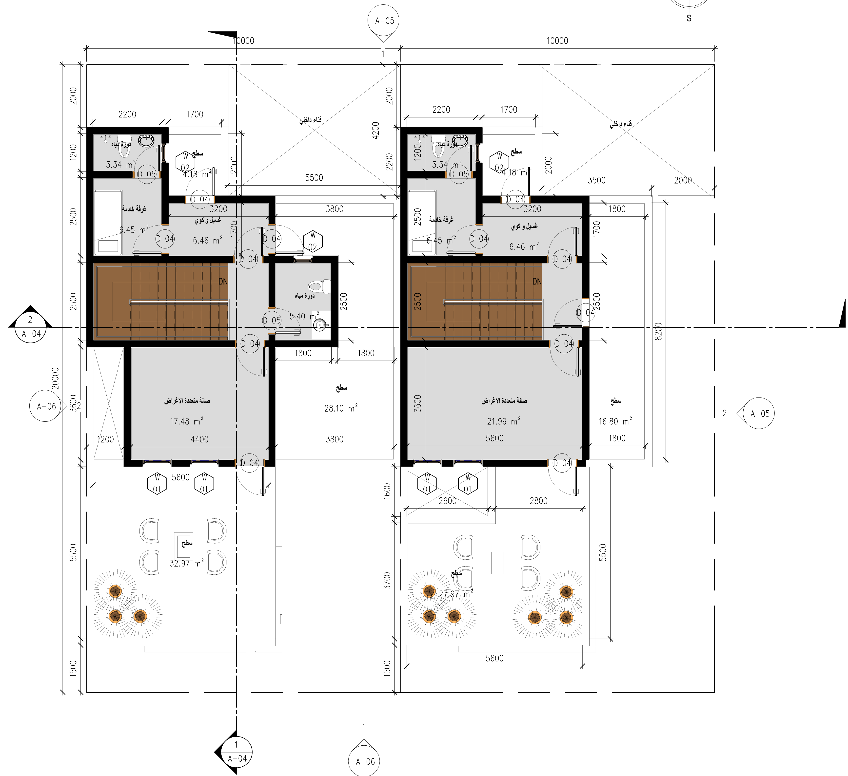
1 ROOF ANNEX FLOOR PLAN 1 : 100
